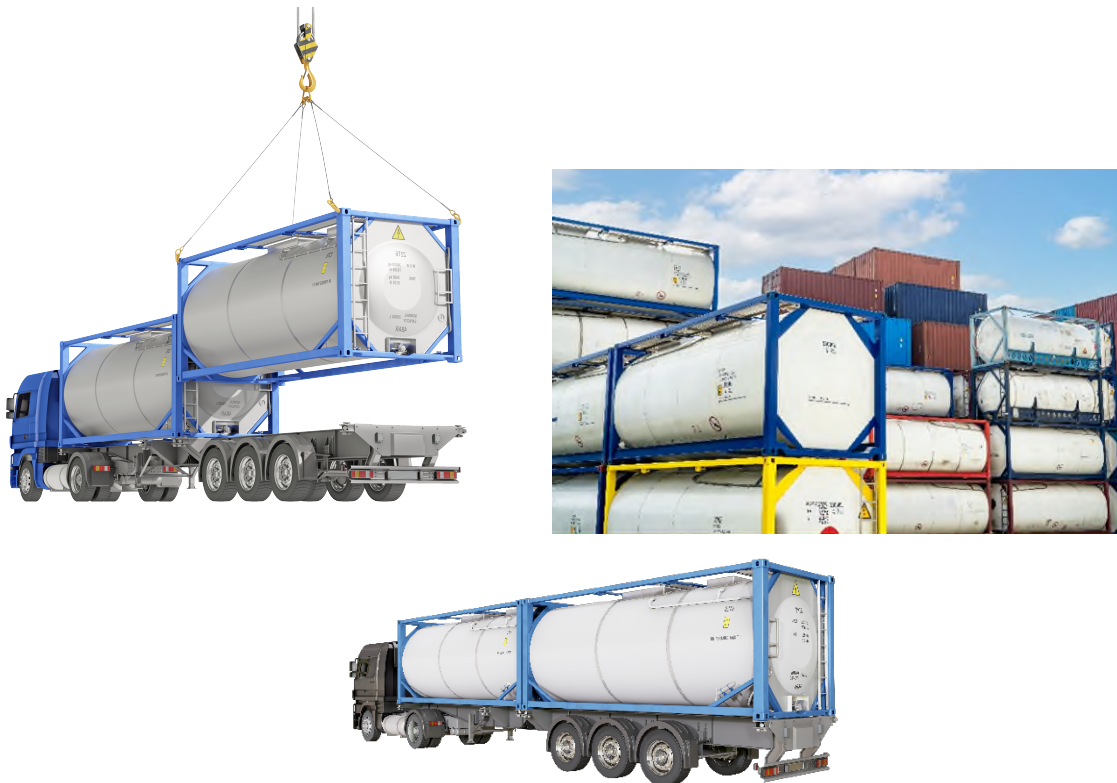
Figure 63: LNG ISO Tanks Stacked and Loaded onto a Standard Container Truck
